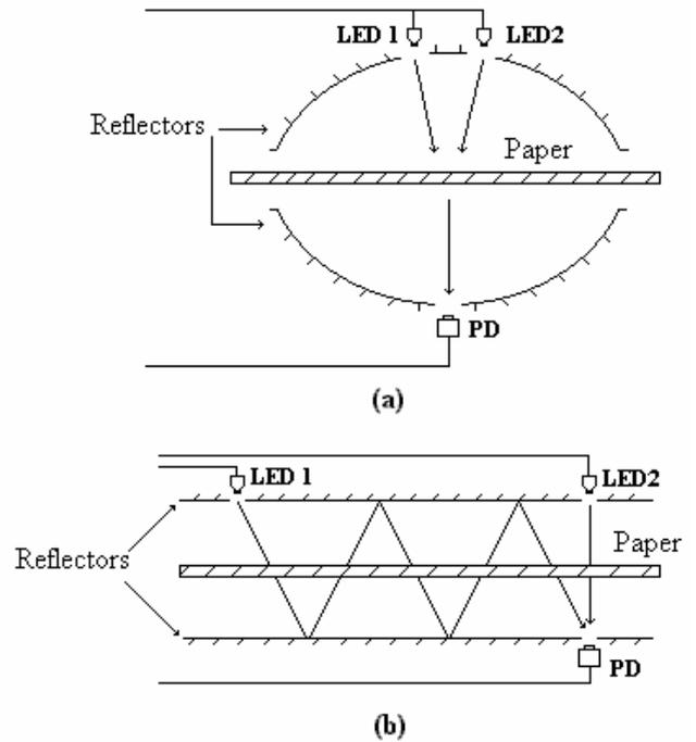
Figure 4 The optical part of a dual- wavelength moisture meter: Parabolic (a) and flat (b) optical reflectors
