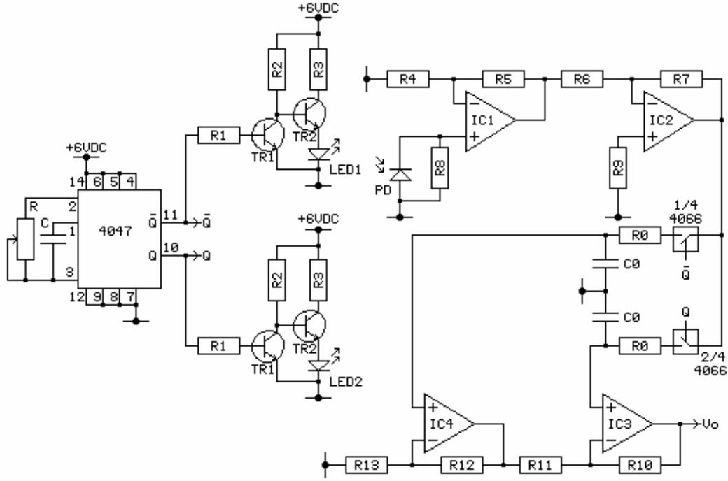
Figure 3 The electrical part of a dual- wavelength moisture meter
