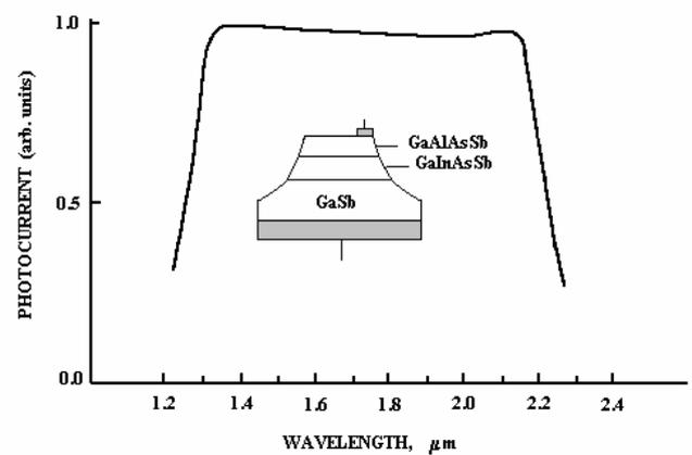
Figure 2 Spectral responses of GaInAsSb/ GaAlAsSb photodiode at room temperature
