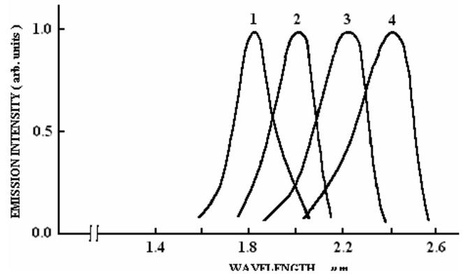
Figure 1 Spectra of emission intensity of GaInAsSb light-emitting diodes at room temperature(See Table 2).
