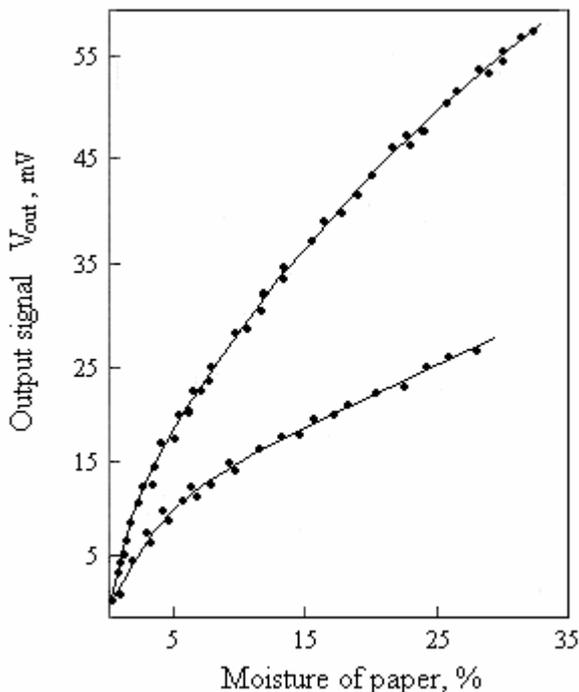
Figure 5 The dependence of moisture content in paper on output signal: 1) with a parabolic and 2) with a flat optical reflectors
