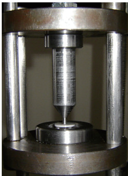
Fig. 1. Placing test specimen on the supporting balls of the tension-compression machine.
