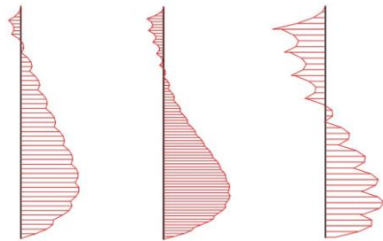
Figure 13. Resultant bending moment on the facing, a. GT, b. GG and c. SS
