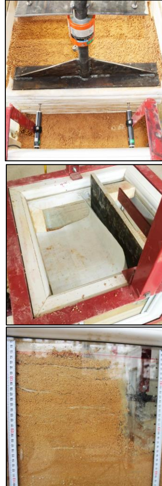
Figure 5. Geotextile reinforced slope (GT), before, pending and after test
