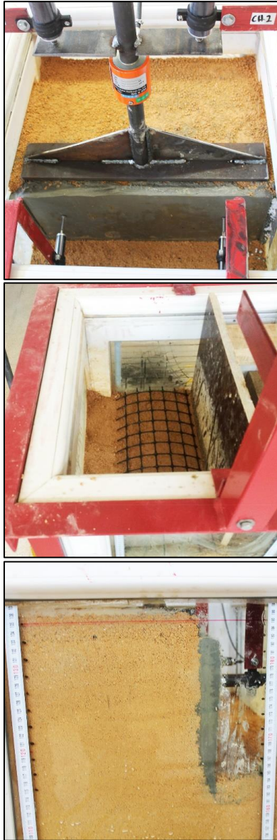
Figure 6. Geogrid reinforced slope (GG), before, pending and after test
