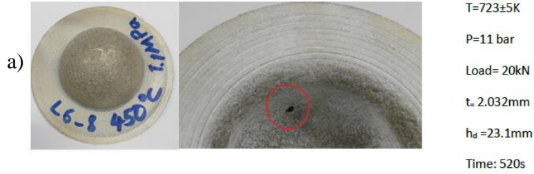
2 nd Specimen (6.9) for replication under the conditions T=723\pm 5K , P=11 bar
