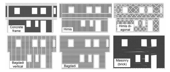
Figure 14. Types of modeled structures
