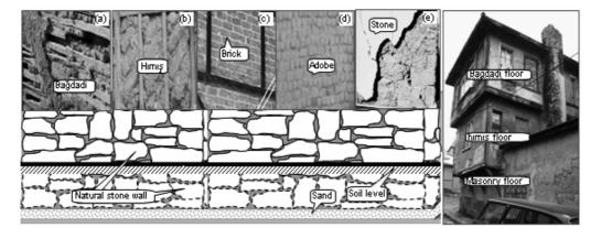
Figure 3. Systems of foundation and kinds of wall
