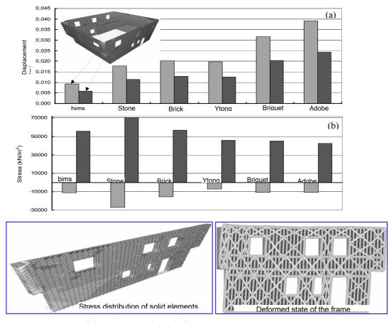
Figure 12. Results of the analyses of Himis frame
