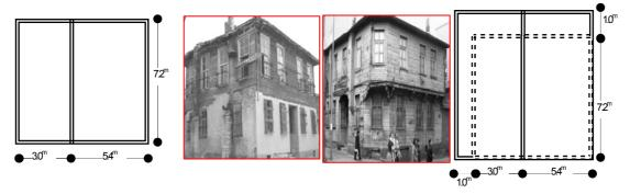
Figure 9. Plan with overhang and without overhang
