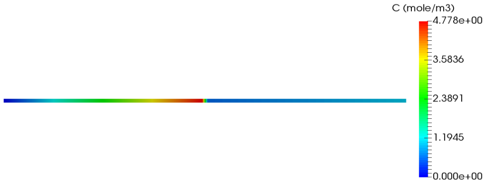
Figure 3.3: Final concentration distribution in computational domain for the 1-Dimensional mass transfer problem
