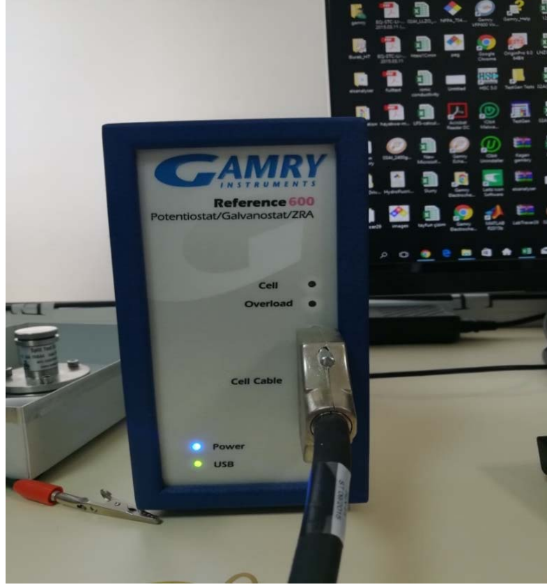
Görsel 2.4. Gamry Instruments Referance 600 model empedans cihazı
