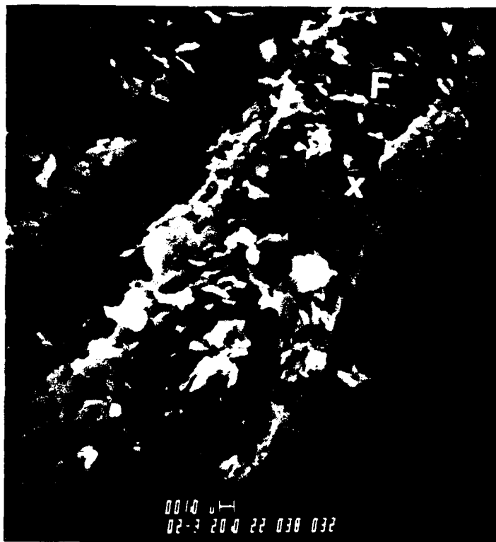
Figure 5.17. SEM Micrograph of Municipal Sludge + Salt Water Mixed Marine Clay Sedimented Specimens (Magnification: 2000X). F: Fibre (coated by clay particles), X: X-Ray Diffraction Spectrum
