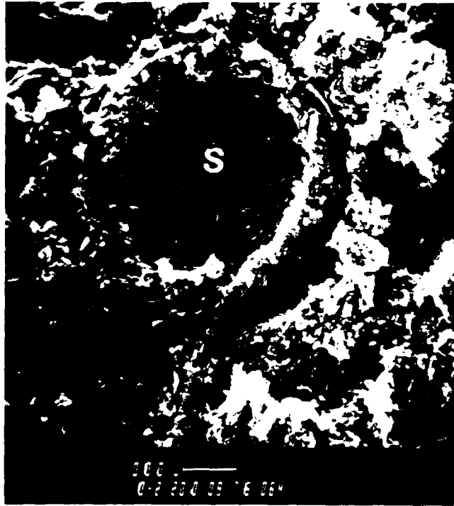
Figure 5.27. SEM micrograph of Salt Water + Crude Oil Mixed Marine Clay Sedimented Specimens (Magnification: 1000X). S: Spherical agglomeration
