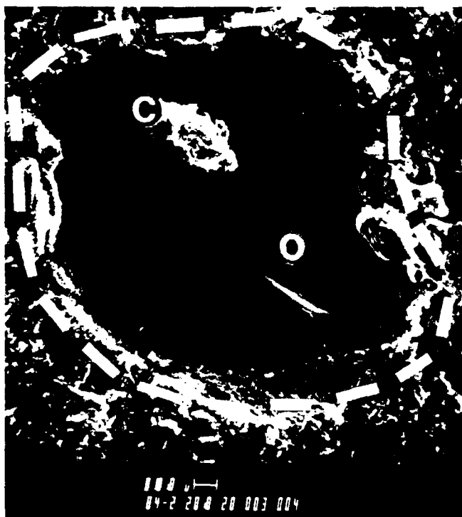
Figure 5.39. SEM micrograph of Salt Water + Crude Oil Mixed Marine Clay Sedimented Specimens (Magnification: 400X). C: Clay particle, O: Oil Surface
