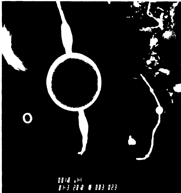
Figure 5.46. SEM micrograph of Salt Water + Crude Oil Mixed Marine Clay Sedimented Specimens (Magnification: 1000X). O: Oil Surface
