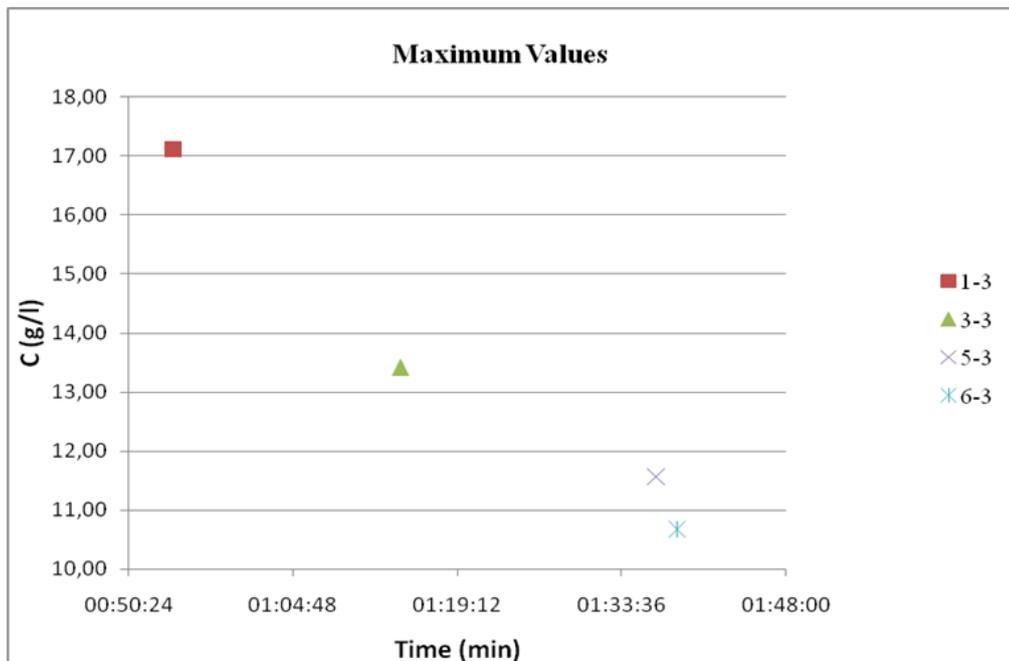
Figure 8. Maximum concentrations and their arrival time for the points on the line 1-3
