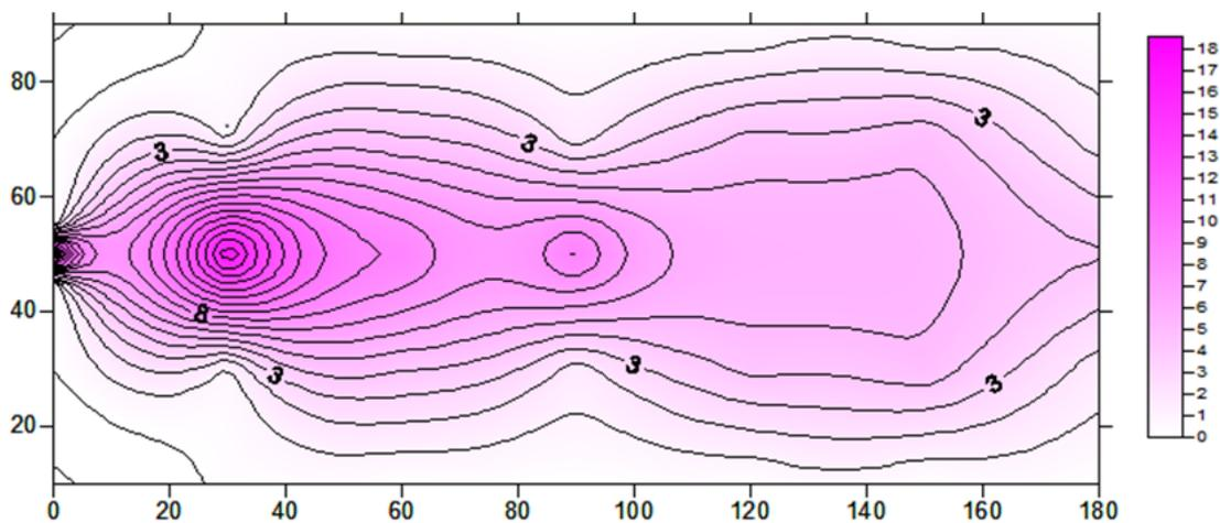
Figure 10. Concentration distribution 55 minutes after the injection
