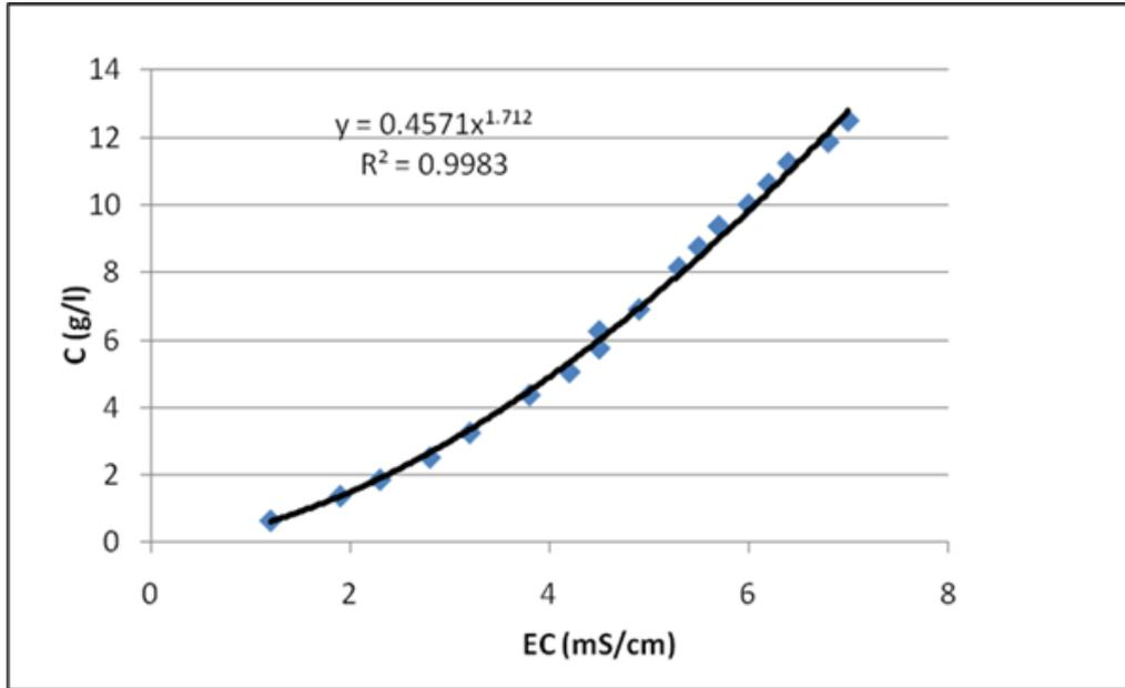
Figure 3. Calibration curve (Concentration versus electrical conductivity)
