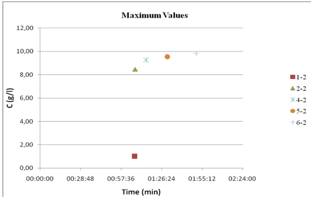
Figure 7. Maximum concentrations and their arrival time for the points on the line 1-2
