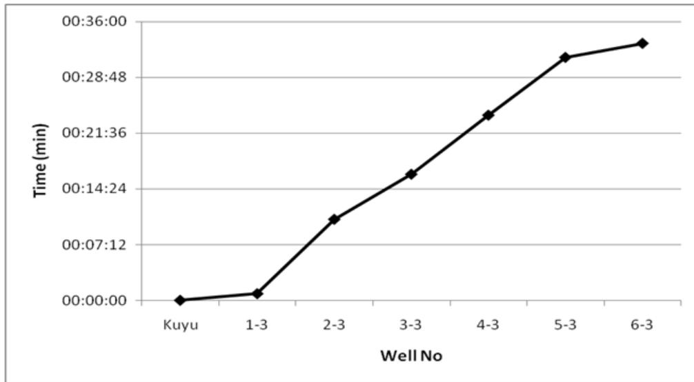
Figure 9. Travel times of the tracer along the axis (line 1-3)
