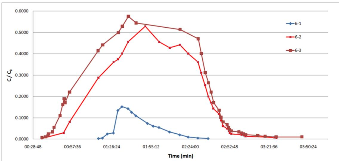
Figure 6 Breakthrough curves in transversal direction
