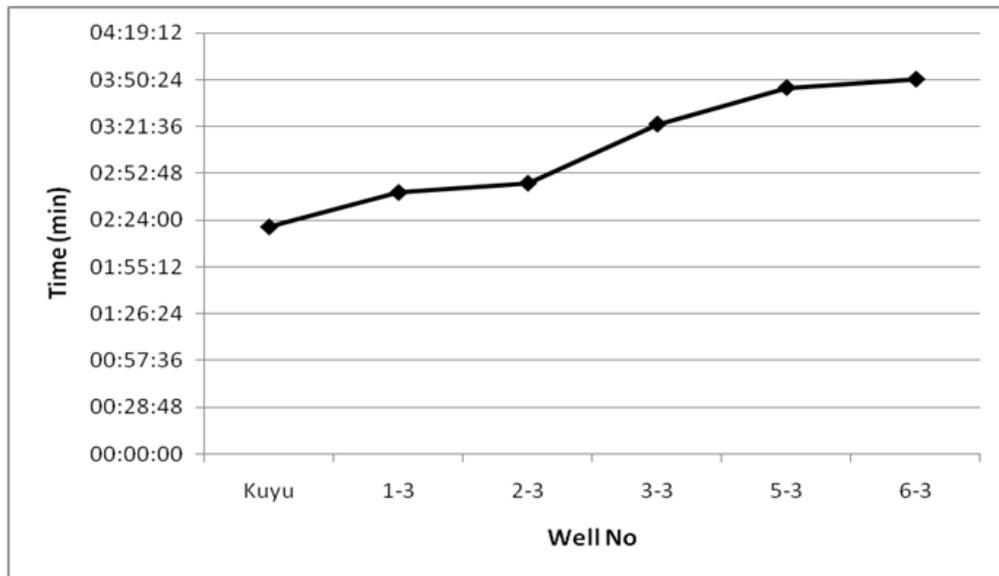
Figure 12. Leave times of the tracer
