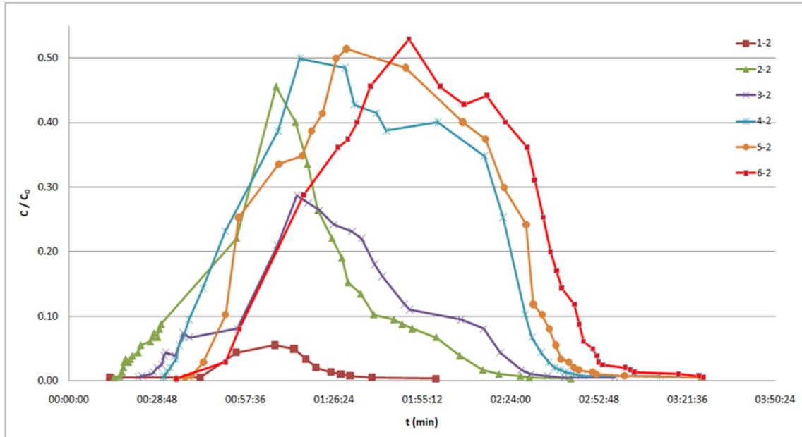
Figure 5. Breakthrough curves in longitudinal direction along the line 2-2
