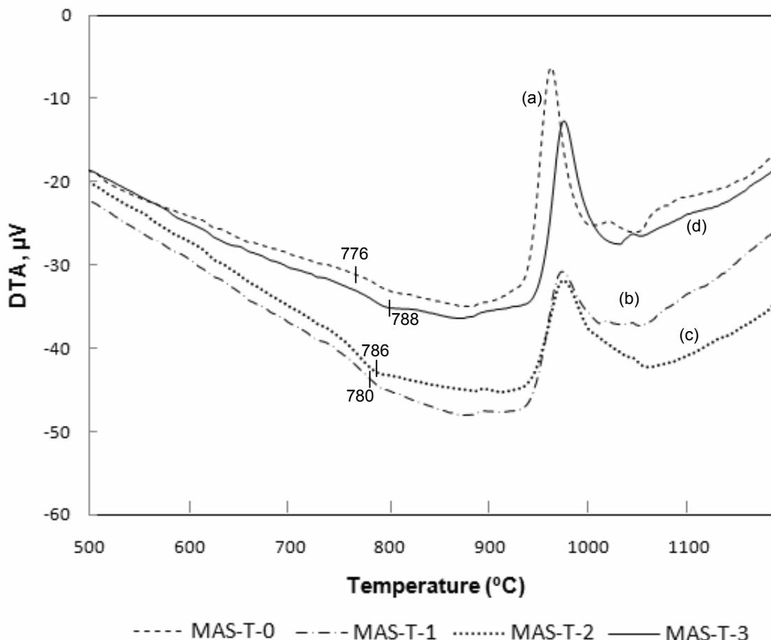
Figure 4. DTA curves of (a) pure, (b) 1%, (c) 2% and (d) 3% B<sub>2</sub>O<sub>3</sub>-doped cordierite glasses
