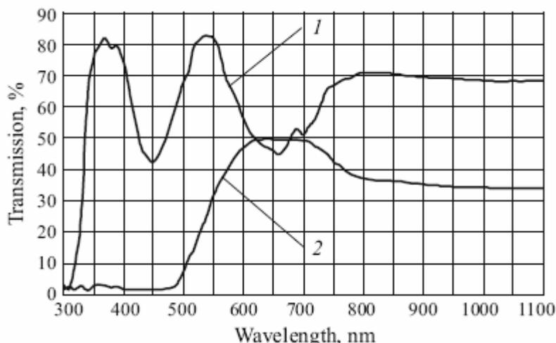
Figure 1. Transmission spectra of green (1) and brown (2) container glasses (Zhernovaya et al, 2007)
