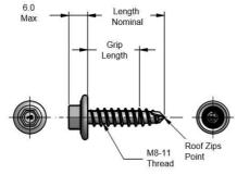
Fig. 4 Screw section detail
