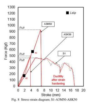
Contemplating the results, it is clear that the capacity of screws both in tension and compression are slightly different from the strength capacity of both used adhesive. The significant difference occurs in the stroke, it is informed in Fig. 10. As information, S1, S2, and S3 showed ductility after strain hardening which are different from the configuration of ASK and A3M with no condition after strain hardening.
