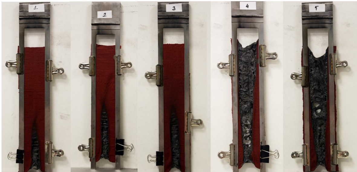
Fig. 5. Vertical flammability test results of the samples
