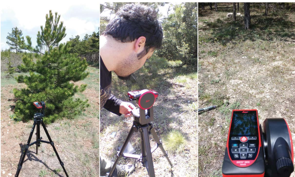
Figure 4. Ground measurements were taken with a laser distance metre.
