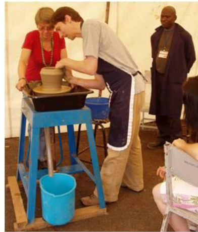
Picture 12: Treadle Wheel Used in Kenya
